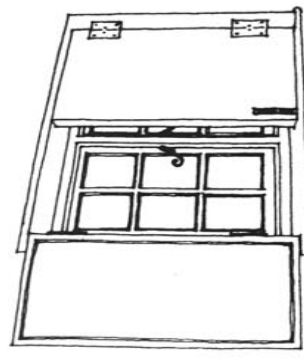
Close-fitting Shutters; image from Eco-Renovation
