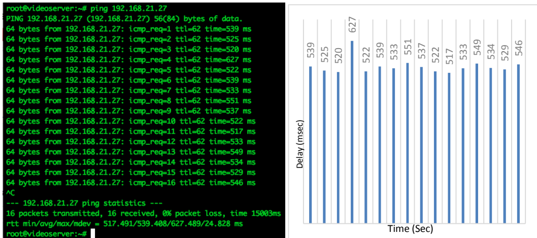
Figure 122. ICMP RTT to the video server over the satellite link
