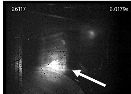
Fig. 11. Example of Oport fast camera view of the SPI fragment interaction with the plasma. The arrow shows the shattered pellet trajectory with the inner wall on the left.
