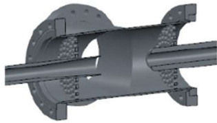
FIG. 2. The microwave cavity implemented for both JET and KSTAR SPI system with perforated screens to enable efficient pumping while screening out the microwaves.
