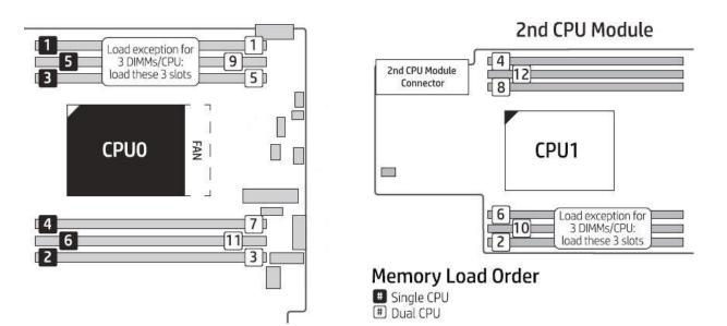
Supports up to 768 GB DDR4-2933 ECC RAM\* (transfer rates up to 2933MT/s) and 384 GB DDR4-2666 ECC **Maximum Memory** RAM (transfer rates up to 2666MT/s). **Memory Configuration** Only Registered ECC DIMMs are supported. (Supported)
