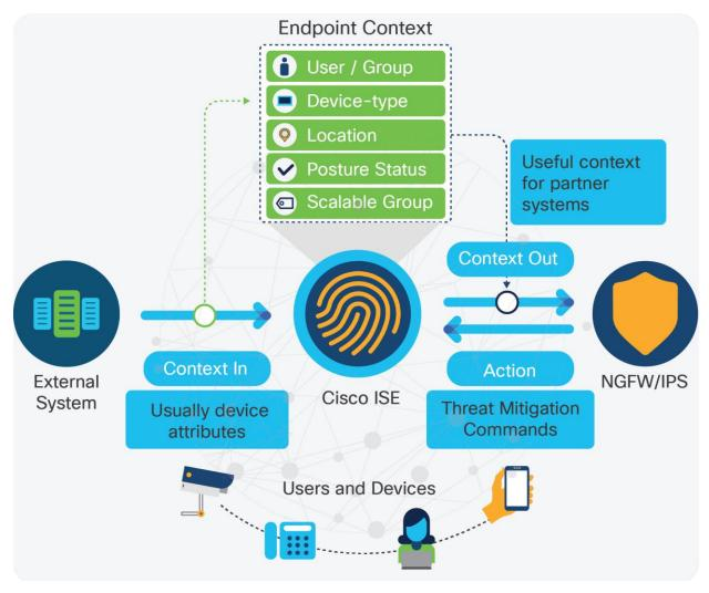
The context exchange between the platforms can be done via Cisco<sup>®</sup> pxGrid or REST APIs.
