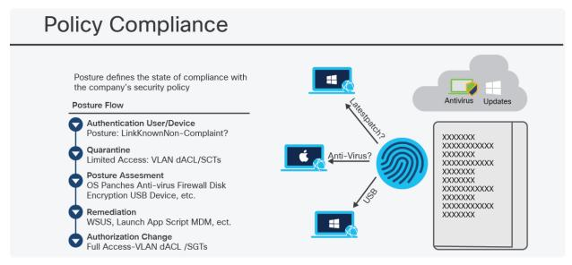
Posture leverages installed and temporal agents looking inside the endpoint to provide assurance that operating system patches, anti-malware, firewall, and more are installed, enabled, and up to date before authorizing the device onto the network.
