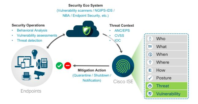
Cisco ISE integrates with security eco-system partners over pxGrid and/or Application Programming Interfaces (APIs) to learn threat level of the endpoints to take mitigation actions.
