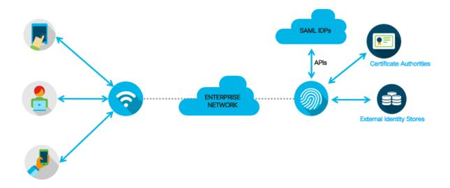
After successful authentication, based on group's information ISE provides the right access the wireless connection, whether the connection is a Passive Identity session (Easy Connect), MAB (MAC Address Bypass) or 802.1x. This can be achieved by assigning the user to a VLAN, DACL, ACL, assign an SGT or SGACL.
