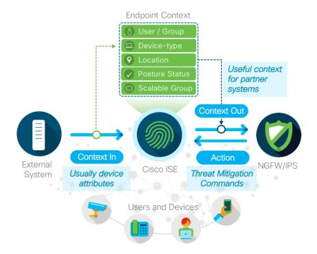
The context exchange between the platforms can be done via Cisco® pxGrid or REST APIs.
