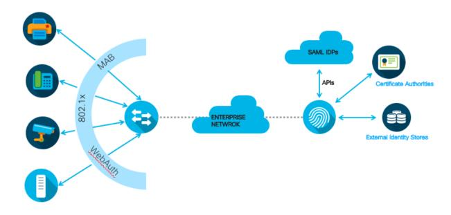
ISE authenticates the users and endpoints via 802.1X, Web Authentication, MAB and other means. ISE can query external identity sources for identity resolutions and apply appropriate network policies by instructing the network devices.
