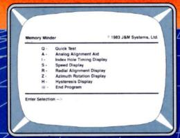
Select any one of seven tests to perform preventive maintenance or to isolate problems. Simple, single-letter commands make MM easy to use! Use MM to align the head, adjust the index hole detector, or adjust the speed.
