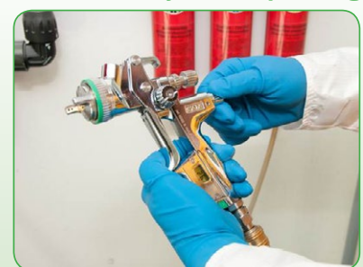
3 Assembly of the air cap - air cap marking must be legible
