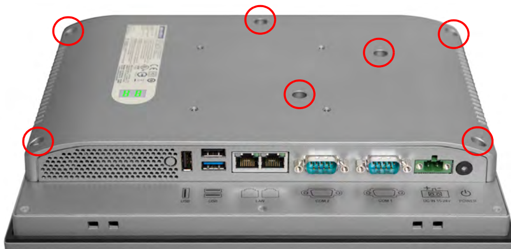
Figure 2.4 Retention screws on rear cover
