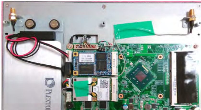
Figure 2.17 Full-size mini PCIe LAN antenna cables
