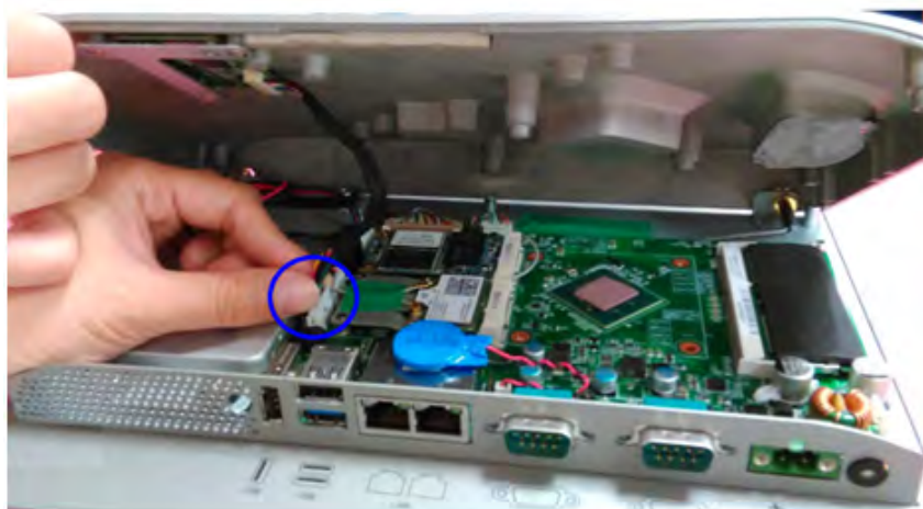
Figure 2.20 Replacing the rear cover
