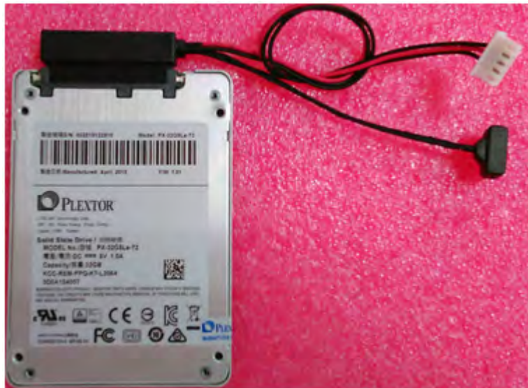
Figure 2.10 SATA cable connected to SATA HDD
