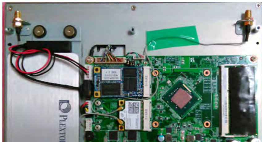
Figure 2.18 Half-size mini PCIe LAN antenna cables
