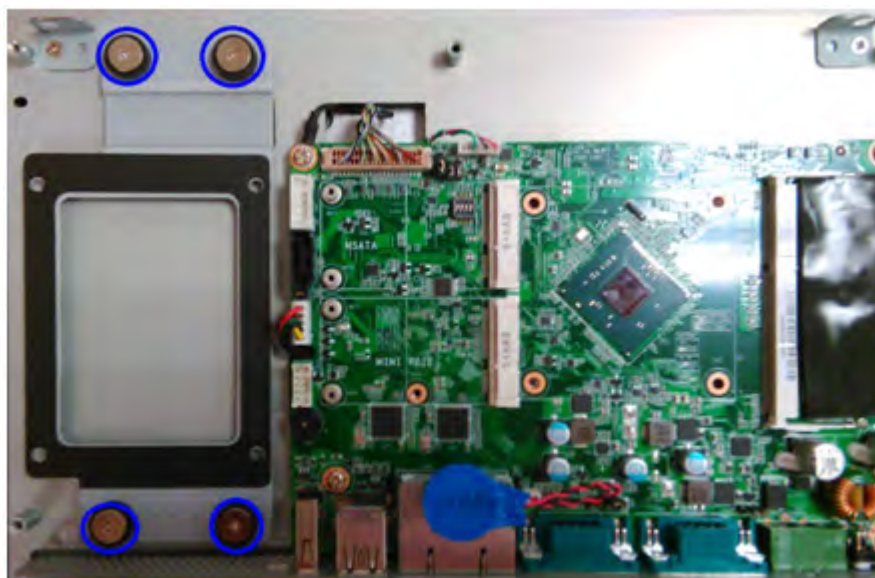
Figure 2.8 Retention screws on HDD bracket
