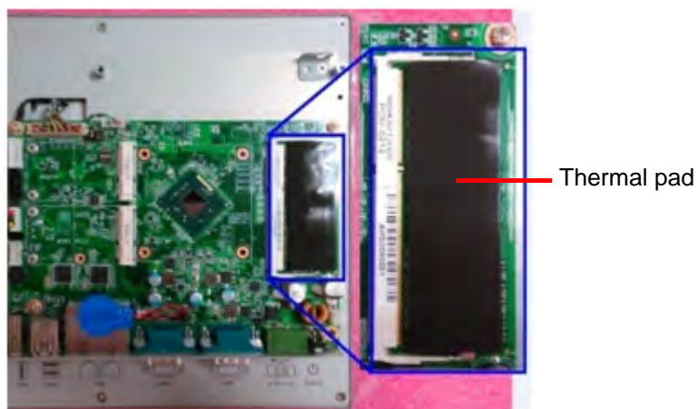
Figure 2.7 Thermal pad placed on the memory card
