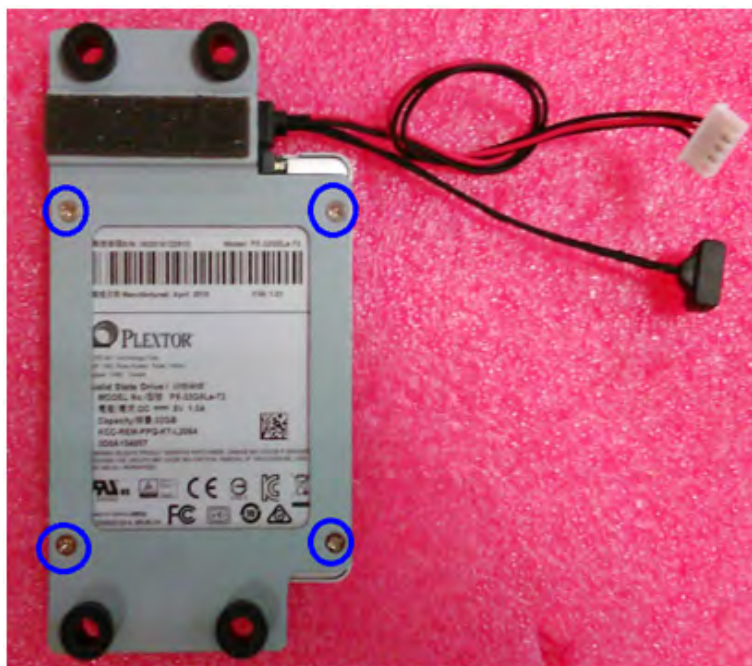
Figure 2.11 Secure SATA HDD with screws
