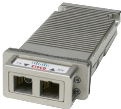
Figure 13. Cisco 10-Gbps Ethernet X2 Transceiver
