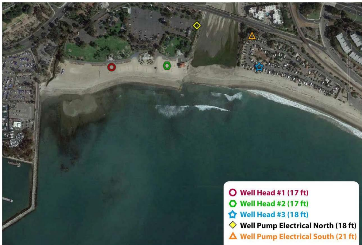
Figure 4.8-1: Critical Shore-front Infrastructure Locations for the Doheny Desalination Project
