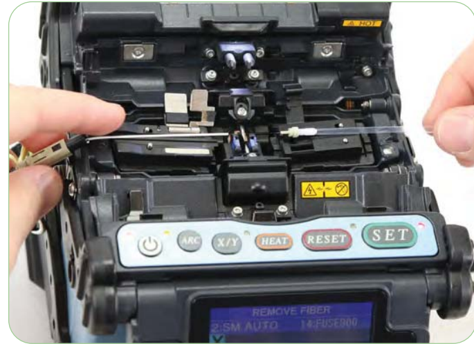
Splicing a FUSEConnect ST Connector
