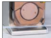
Head allows alternate placement of tubing.
