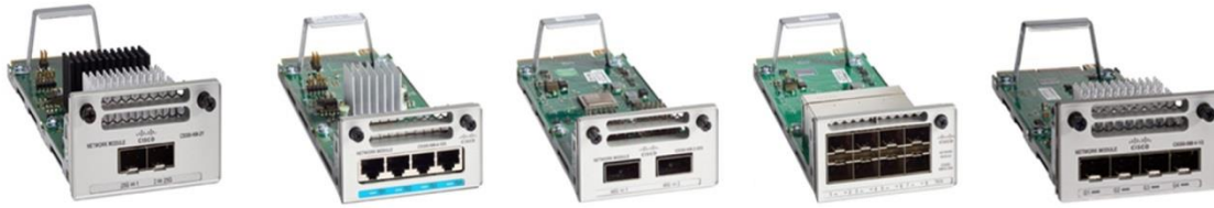
Figure 2. Cisco Catalyst 9300 Series Network Modules
