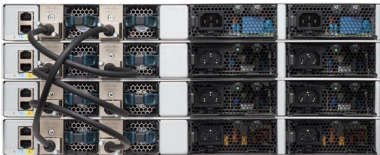
Figure 4. Cisco Catalyst 9200 Series Switch stacked units
