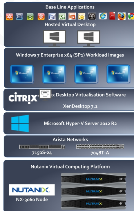
Figure 2. Citrix Validated Solution Stack depicting HVD Workloads
