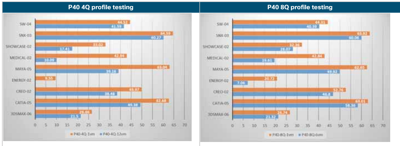
Figure 103. SPECviewperf results for P40 4Q and 8Q profile tests: Single virtual machine versus maximum host density based on profile size
