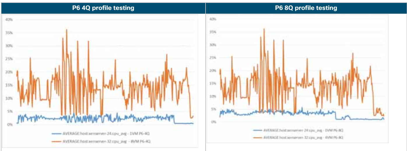
Figure 107. Cisco UCS B200 CPU utilization results for SPECviewperf P6 4Q and 8Q profile tests: Single virtual machine versus maximum density
