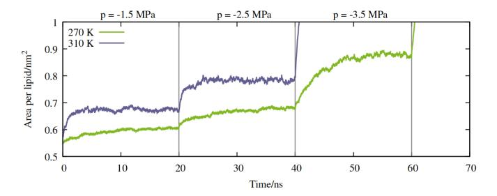
Figure 2: Expansion of the mixed monolayer during sequential pulling simulations, with increasingly negative pressure p, at  $T=270~{\rm K}$  (green) and 310 K (blue).
