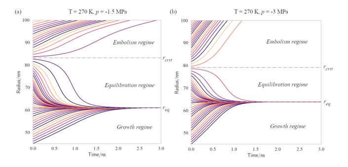
Figure 6: Bubble dynamics produced by integration of the Rayleigh-Plesset equation (Eq. 6), assuming  $N_{\text{lipids}} = 10^5$ , T = 270 K, and (a) p = -1.5 MPa, or (b) p = -3 MPa. Each panel contains 55 scans initialised at radii equally spaced between 45 and 100 nm. Further details in main text and Methods.
