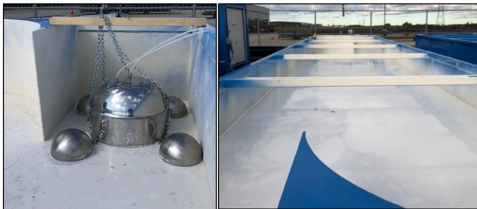
Figure 3 – Open tank FRB system using a flux chamber (left) and buoyant photocatalyst (right)
