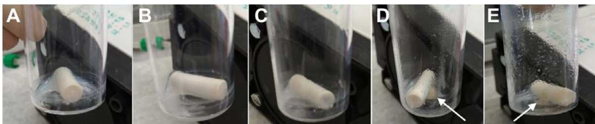
Figure 5. Bottom of the glass vials and magnets after synthesis of gelatin nanoparticles under stirring from the mixtures of gelatins A with bloom values of 300 and 62. A - A300:A62=4:0; B - A300:A62=3:1; C - A300:A62=2:2; D - A300:A62=1:3; E - A300:A62=0:4. Large gelatin aggregates are labeled with arrows.
