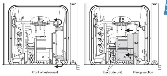
Fig. 7-41 (The figure shows the LCMS-8040.)
