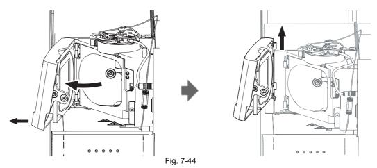
3 Remove the ESI and APCI probes from the instrument.
