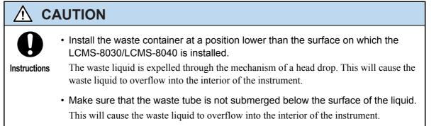
Prepare a waste container of an appropriate capacity (diameter of mouth: 29 to 31 mm) and place this container at a position lower than the instrument (e.g. on the floor).
