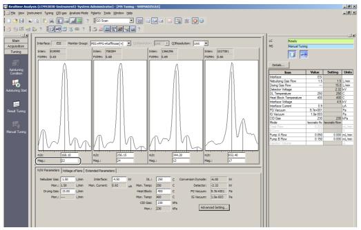
Move the mouse cursor into the ion observation panel and double click to display the data standardized at the maximum intensity.
