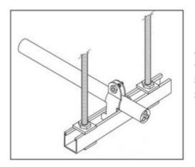
**A. Trapeze-type Supports** – When the cable is installed on/from trapeze-type supports, the trapeze-type supports shall be secured from the surface of the floor. The supports shall be spaced a maximum of 5 feet on center.
