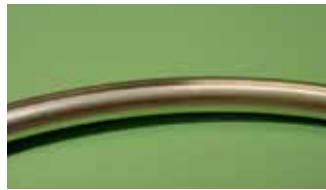
Figure 2: Parker Hannifin's Silver-Indium diffused plating
