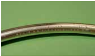
Figure 1: Blisters seen on a standard silver plated seal after 1,000 hours in air at 260 °C (500 °F)
