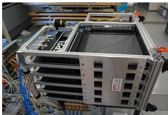
Figure 8: The SciFi tracker detector setup in the lab for cosmic ray test. The active area of a tracker module is 40\ \text{cm} \times 40\ \text{cm} and consists of 5 x y fibre planes.
