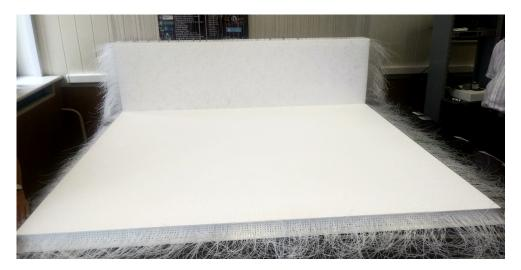
Figure 28: Picture of both Wall ( $15 \times 56 \times 192$  cubes) and Plane ( $192 \times 5 \times 186$  cubes) Prototypes assembled with fishing lines.
