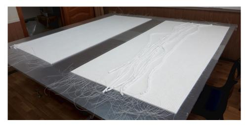
Figure 25: The layer assembly by dividing the cube arrays in two half-planes. Each divided layers consist of 92 cube arrays, and the arrays are aligned by the 1 m long, 1.2 mm diameter spokes inserted through the horizontal holes.
