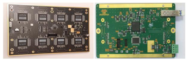
Figure 19: The first FEC (left) and FEM (right) prototypes.
