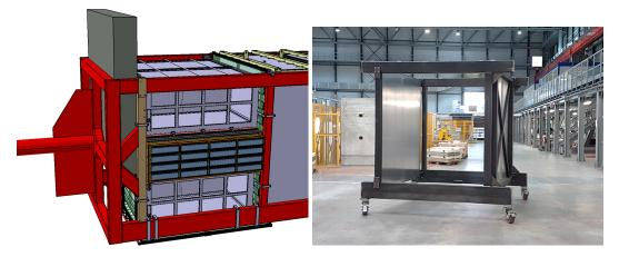
Figure 21: *Left:* CAD sketch of the basket during the ECAL re-installation. *Right:* Photo of the BabyBasket which reassembles the same geometry as the ND280 basket.
