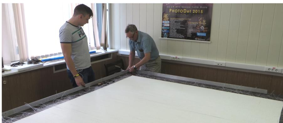
Figure 26: The  $192 \times 5 \times 184$  Plane Prototype assembly using the right angle, aluminum profile. The height of the corner is equivalent to 5 Super-FGD cubes.
