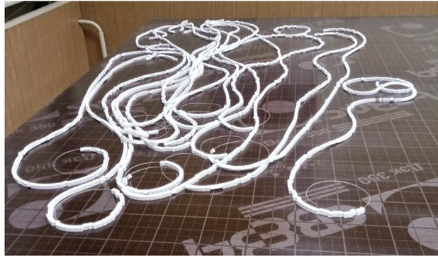
Figure 24: Picture of assembled 192-cube arrays with fishing lines.
