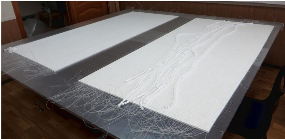
Figure 25: The layer assembly by dividing the cube arrays in two half-planes. Each divided layers consist of 92 cube arrays, and the arrays are aligned by the 1 m long, 1.2 mm diameter spokes inserted through the horizontal holes.
