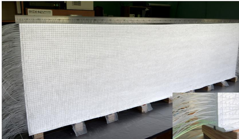
Figure 31: Wall Prototype with sagging depth of 10 mm. Inserted picture shows the WLS fibers inserted in the lowest layer of the Prototype.
