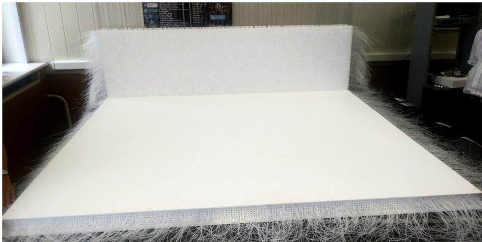
Figure 28: Picture of both Wall ( $15 \times 56 \times 192$  cubes) and Plane ( $192 \times 5 \times 186$  cubes) Prototypes assembled with fishing lines.
