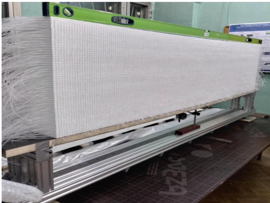
Figure 4: 56 narrow-size layers of cubes assembled together into a tower for the sagging measurements.
