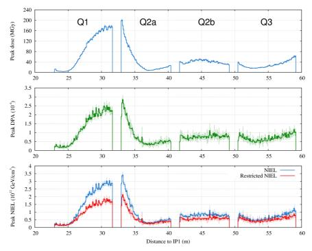
4.1 Radiation map for the Interaction Region (IR) Quadrupoles [1] for the innermost 3 mm for the unshielded case with an integrated luminosity of 3000 nb<sup>-1</sup>
