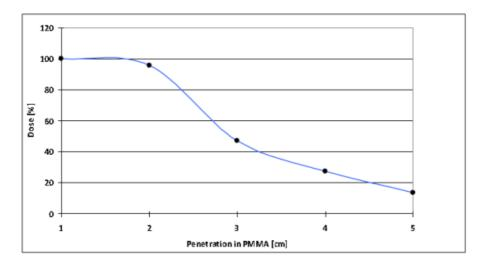
Figure 5.2 Measured depth-dose curve of "12 MeV" structure - confirmed energy: 7 MeV - 8 MeV.
