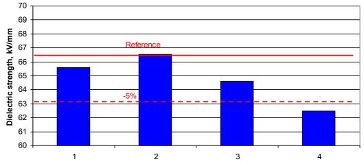
Figure 6.7. Electric strength test results of 550 µm thick G10 laminate, reference data [13]
