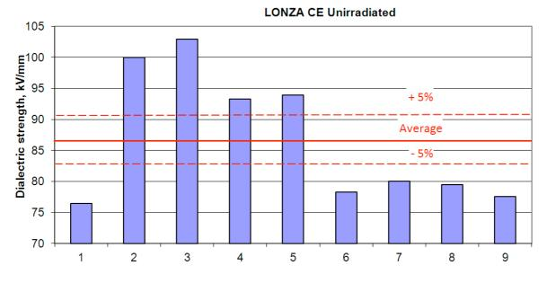
Figure 6.10. Unirradiated LONZA CE electrical breakdown strength
