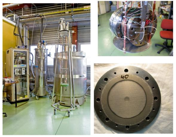
Figure 8.4. Superfluid helium HeII pressurized test cryostat at CEA Saclay
