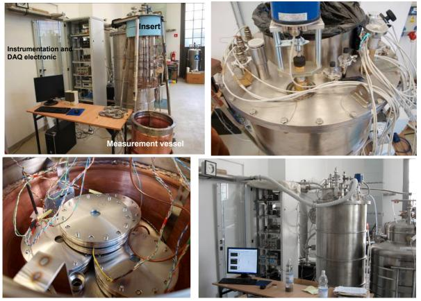
*Figure 8.3. Superfluid helium test cryostat at Wroclaw University of Technology* For the thermal measurement purpose CEA-Saclay used the NED cryostat, which design is presented in [10,11]. The pressurized superfluid test vessel dimensions allow simultaneous
