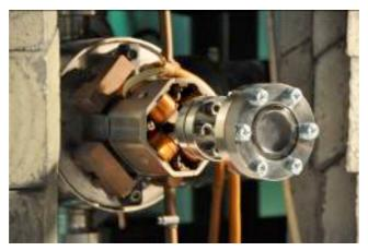
Figure 5.10. 0.2 mm thick Ti accelerator window.
