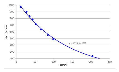
Figure 5.4 Dose rate variation as function of the distance from the radiation source in air for the 6 MeV structure, PRR = 76.4 Hz. Accelerator parameters <u>not optimized</u>. [4]
