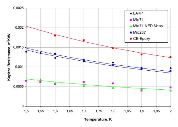
Figure 8.6. Kapitza resistance measurements results
