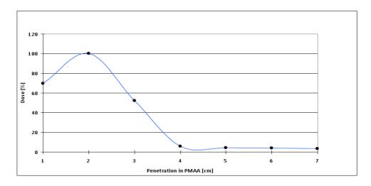
Figure 5.3 Measured depth-dose curve of "15 MeV" structure - confirmed energy: 10 MeV - 11 MeV.
