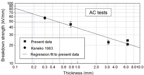
Figure 6.5. Rreference data for G10 laminate tested with AC voltage [13] Figure 6.6 and 6.7 present the 190 µm and 550 µm thick G10 electric strength test results.
