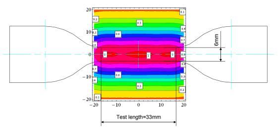
Figure 5.13. Irradiation dose distribution for mechanical specimen irradiated in 3 locations. Distance between irradiation spots d=18 mm.
