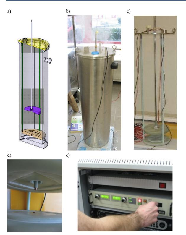
Figure 6.1. Electrical test stand view, a) electrical cryostat conceptual design, b) the cryostat view, c) the cryostat insert view, d) the test part of the insert view, e) SL600 type Spellman High DC Voltage source
