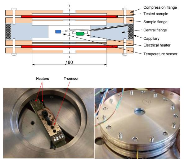
Figure 8.1. Sample holder for thermal tests of irradiated samples
