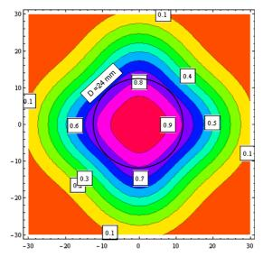
Figure 5.12. Irradiation dose distribution for specimen irradiated in 5 locations. Distance between irradiation spots d=15 mm.
