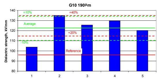
Figure 6.6. Electric strength test results of 190 µm thick G10 laminate, reference data [13]
