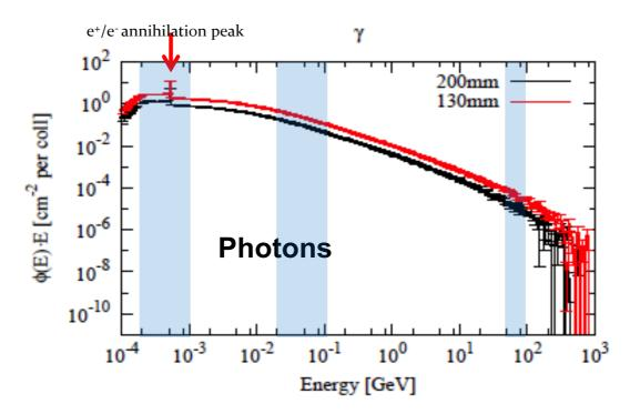
Figure 4.2 Photon spectrum on the inner coil of Q2a at the peak location for 2 different magnet aperture diameters [2]
