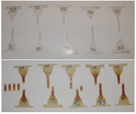
Figure 7.6. View of unirradiated and irradiated LARP samples after the UTS test
