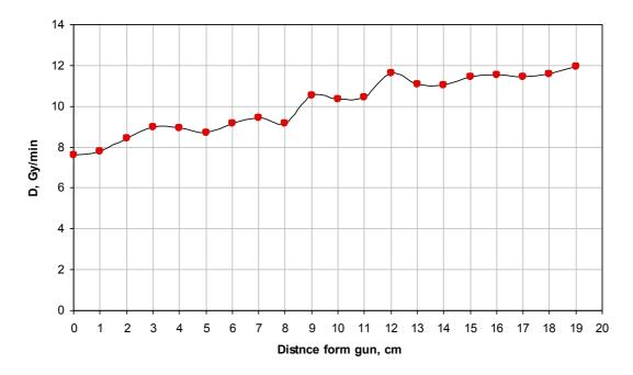
Figure 5.5 Dose rate variation as function of the distance form the radiation source in air for the 15 MeV structure, PRR = 5 Hz. Accelerator parameters not optimized.[5]
