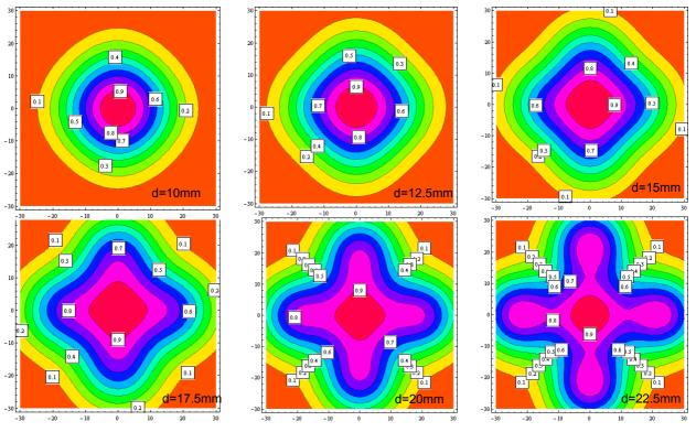
Figure 5.11. Irradiation dose distribution for specimen irradiated in 5 locations: central, top, bottom, left and right from the specimen centre, for different distance d from the spot's centre
