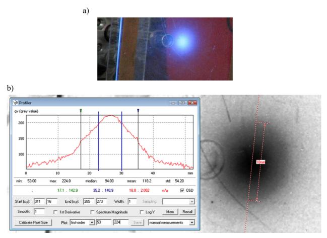
Figure 5.6. Measurement of the beam diameter for the 6 MeV structure, a) projection of the beam on a PMMA plate, b)determination of the beam intensity distribution with picture color analyses
