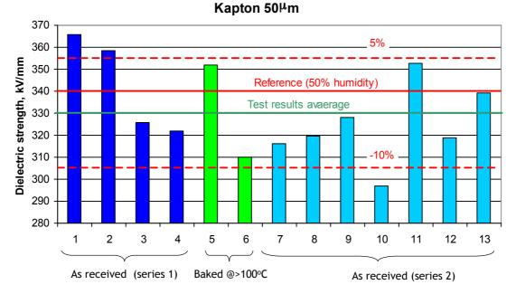
Figure 6.3. Reference electrical tests results for Kapton 50 µm, reference data [12]. AC measurements scaled to DC equivalence.
