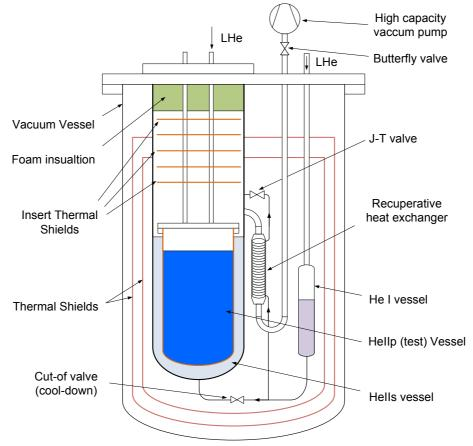
Figure 8.2. Superfluid helium test cryostat flow scheme
