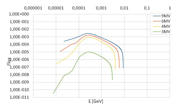
Figure 5.1 Typical spectrum of brehmstrahlung radiation induced by: 9 MeV electrons (blue), 6 MeV electrons (red), 4MeV electrons (yellow) and 3 MeV electrons (green).[3]
