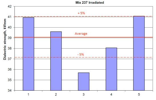
Figure 6.13. Irradiated Mix 237 electrical breakdown strength
