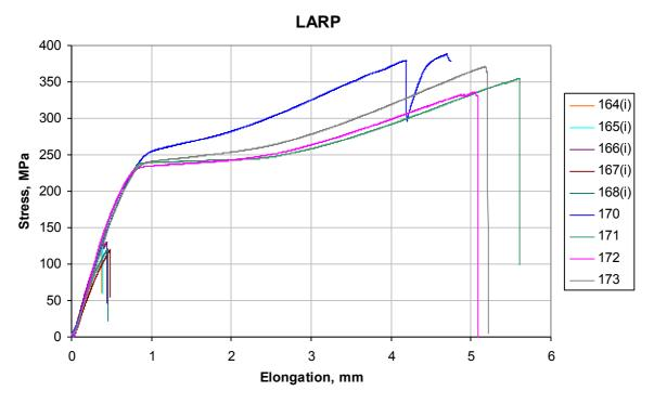
Figure 7.3. UTS test results for unirradiated and irradiated (i) LARP samples
