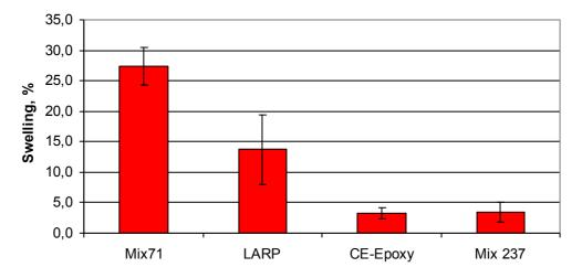
6.16. Insulation materials swelling due to 50MGy electron irradiation at 77K
