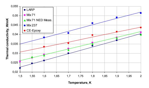
Figure 8.5. Thermal conductivity of the tested samples
