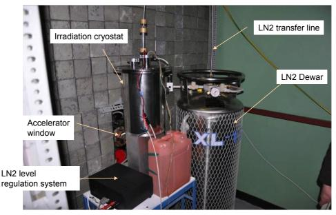
Figure 5.8. Irradiation set-up installed on the accelerator site in NCBJ, Poland.
