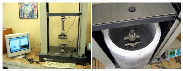
Figure 7.1. View of the mechanical test set-up (left) and its up-date layout with the cryogenic vessel.
