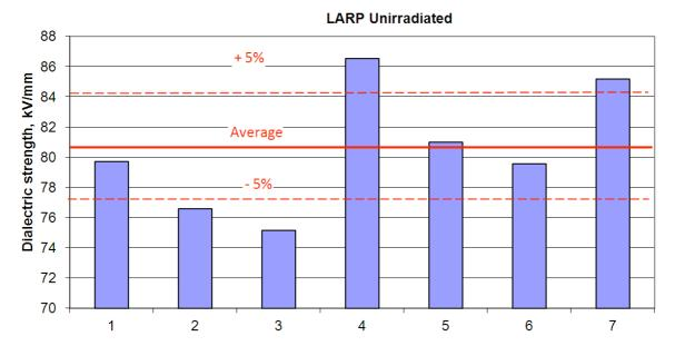
Figure 6.8 Unirradiated LARP electrical breakdown strength
