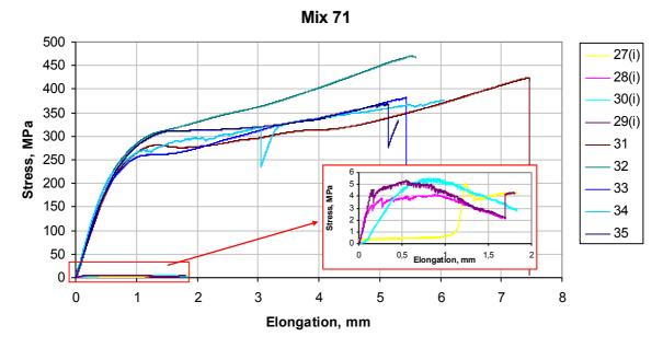
Figure 7.5. UTS test results for unirradiated and irradiated (i) Mix71 samples
