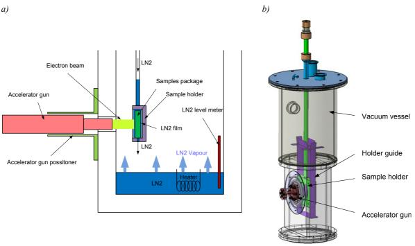
Figure 5.7. Irradiation cryostat, a) scheme, b) view of conceptual design.
