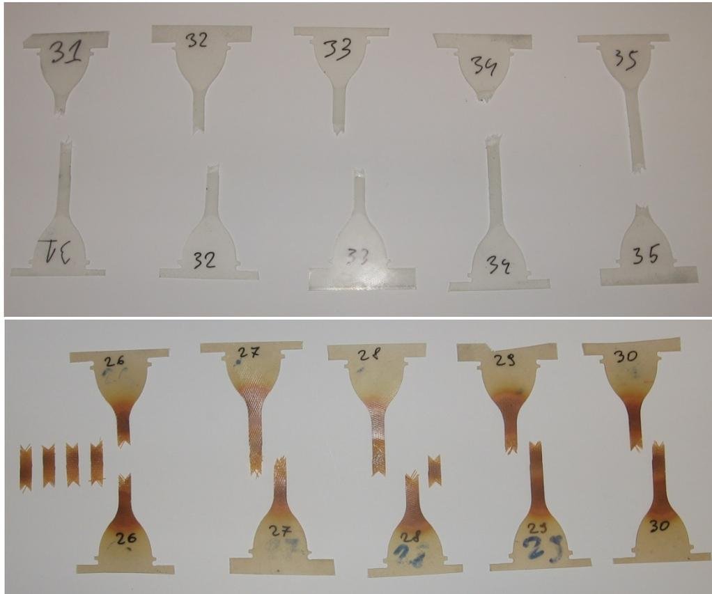
Figure 7.6. View of unirradiated and irradiated LARP samples after the UTS test
