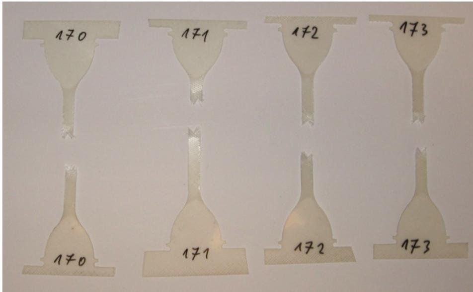
Figure 7.4. View of unirradiated (lower) and irradiated (upper) LARP samples after the UTS test
