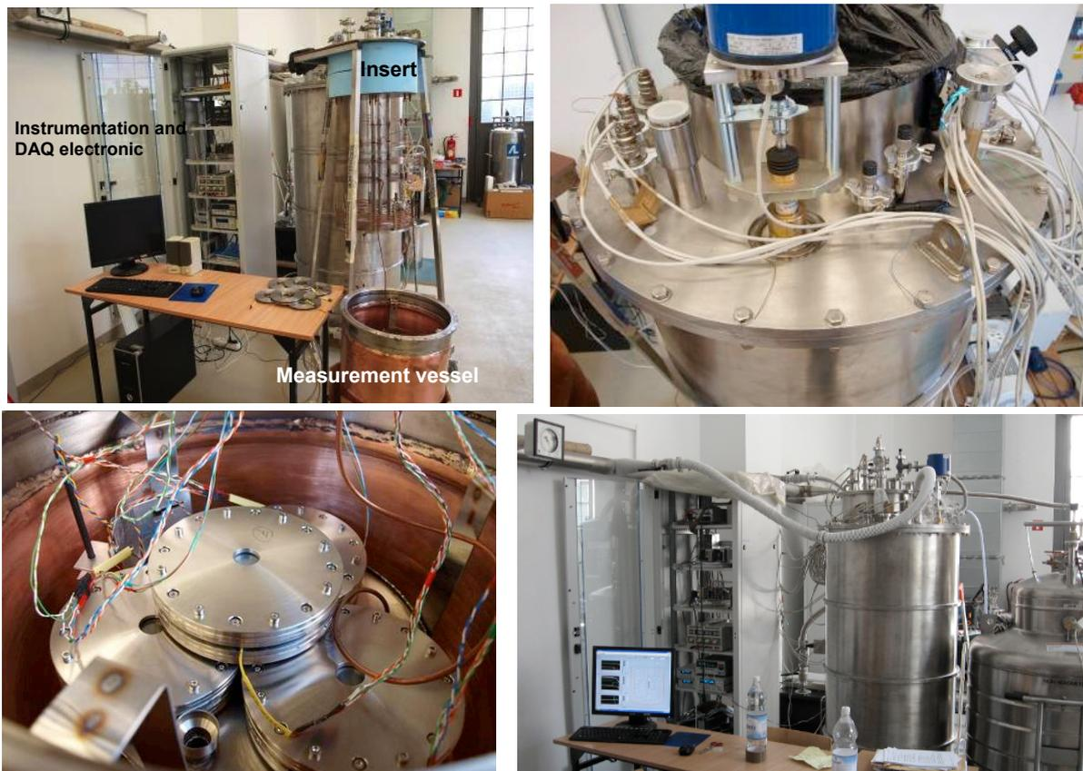
Figure 8.3. Superfluid helium test cryostat at Wroclaw University of Technology
