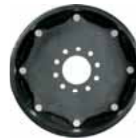
Hub Adapter MSPN 04630 CAI 336820 12 mm thick 1015 carbon steel / reversible 3.68" (93.5 mm) center dia. 10 x 140 mm bolt pattern 0.63" (16 mm) bolt holes, tapered Fits some truck mounted forklifts
