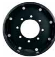
Hub Adapter MSPN 47868 CAI 291074 12 mm thick 1015 carbon steel / reversible 6.0" (152.4 mm) center dia. 8 x 8.0" bolt pattern 0.67" (17 mm) bolt holes, tapered Use adapter to change offset on 8 x 8.0" standard filmet size
