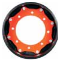
Hub Adapter MSPN 47462 CAI 481115 12 mm thick 1015 carbon steel / reversible 9.0" (228.6 mm) center dia. 8 x 10.75" bolt pattern 0.67" (17 mm) bolt holes, tapered Fits some Bobcat machines
