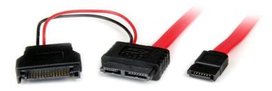
The SLSATAF50CMS 0.5m Slimline Adapter features a (7-pin) SATA female data connection and a SATA power connection on one end, with a slimline Serial ATA female connection on the other, enabling you to connect a slimline optical drive to a SATA controller and power connection.
