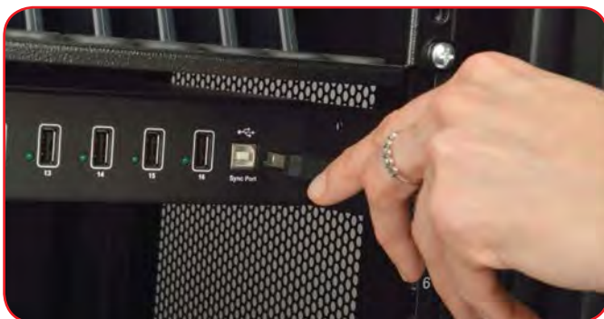
Connect the included USB cable to the sync uplink port and your computer. Cable access allows syncing while the cabinet is locked.
