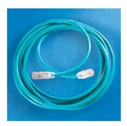
Clarity 6 Modular Patch Cord, blue, 7', Category 6, four-pair UTP stranded 24 AWG PVC/CM, center tuned with Clarity 6 connecting hardware for optimum Category 6 installed performance using Ortronics Paralign 2 pair-positioning technology
