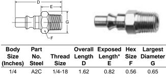
\* This dimension represents portion of nipple that is exposed when nipple is inserted in coupler.
