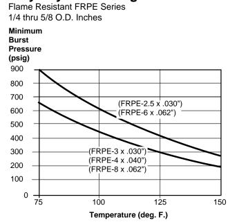
Suggested working pressure of polyethylene is 1/3 of burst pressure at system operating temperature.
