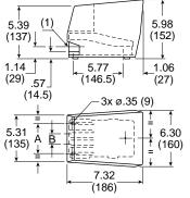
(1) 2 mounting ports for adaptors for conduit fittings (2) 7° operating angle
