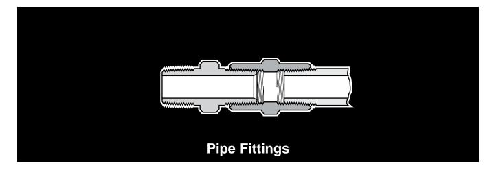
All pipe fitting threads are made to Dryseal standards. Connectors, unions, nuts and extruded elbows and tees are machined from CA 360 or CA 345 brass rod; forged elbows and tees are machined from CA 377 brass.
