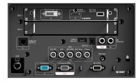
USB connector Type B x 1: for Firmware update, Copy OSD Settings USB connector Type A x 1: for Firmware update, Copy OSD Settings, DC Out 900 mA Monitor out: Mini D-sub 15-pin x 1 Serial: RS-232c x 1 Remote: Stereo mini Wire LAN x 1 etherCON
