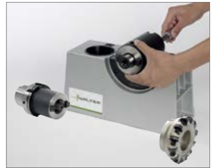
6. Screw the extension and the end mill adaptor together by hand using the socket wrench
