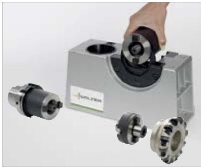
5. Insert the extension into the insert collar
