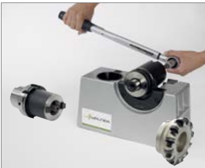
7. Tighten using a torque wrench
