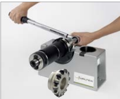
10. Tighten using a torque wrench
