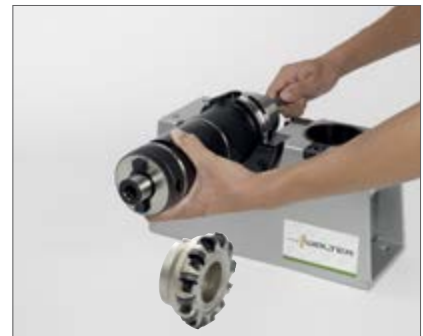
9. Screw the NC tool elements together with the master
