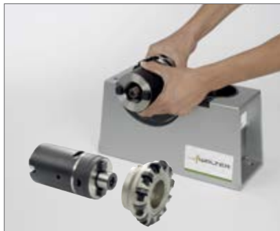
8. Insert the master into the associated flange
