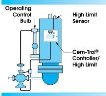
A pilot operated valve can be used with steam as the energy source. Pilot operated valves are not suitable when boiler water is the heating medium.
