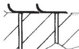
Two sleeves for double seal installation.
