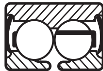
C10 Two Seals Split Inner Ring w/ABS sensor built into seal on one side
