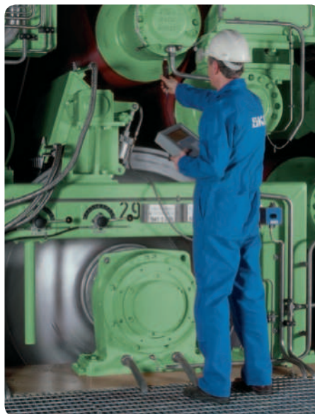
Checking vibration levels
