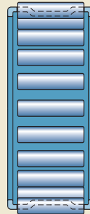
Sheet steel cage of the radial bearing
