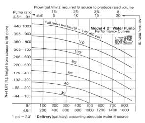
The High Lifter can be used for domestic water pumping, irrigation, range cattle and similar applications. All High Lifter parts are made from stainless steel, Teflon and polyethylene.
