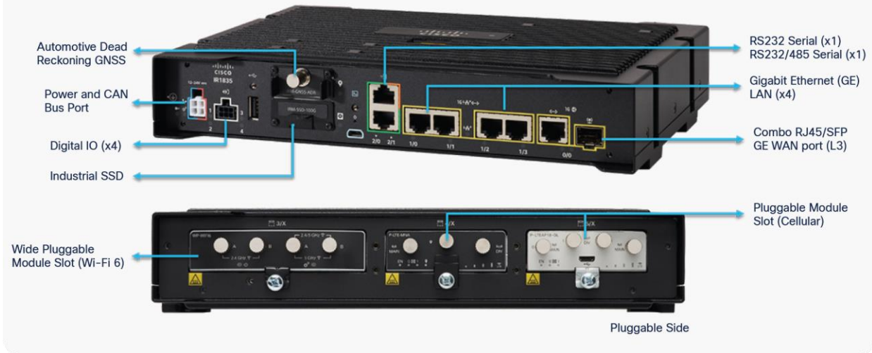
Figure 6. IR1835-K9 interface ports
