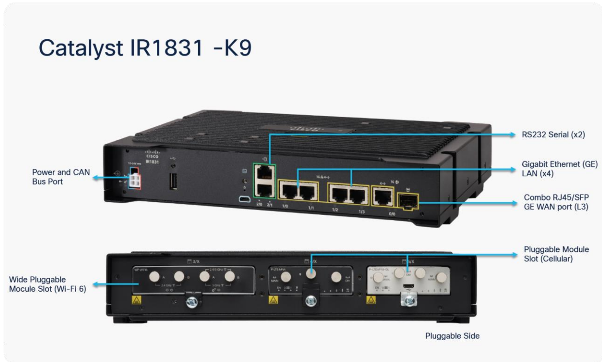
Figure 4. IR1831-K9 interface ports
