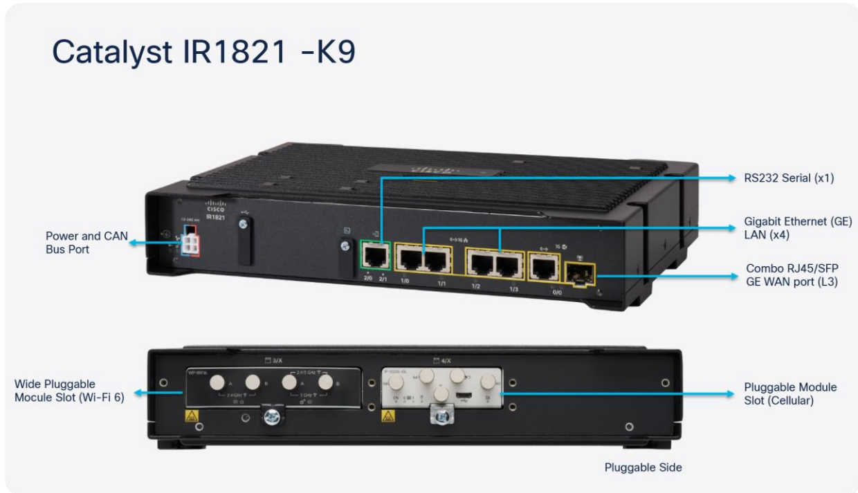
Figure 3. IR1821-K9 interface ports
