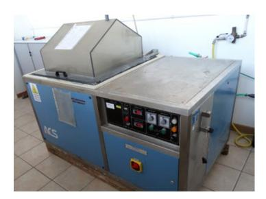
**Accelerated harsh-weather testing** is performed to ensure components under test meet qualification requirements for galvanic corrosion and resistance, resistance to solvents, and S02.
