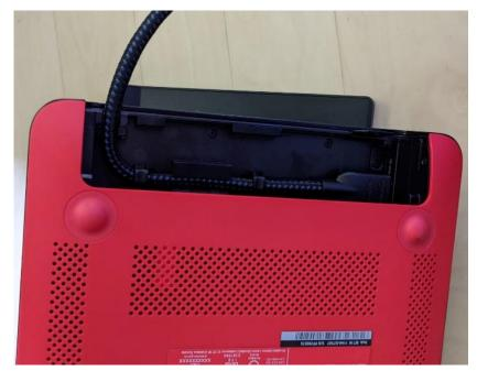
3. On the red side of One Cable, slide the plastic cover down to reveal the blocks of connectors.
