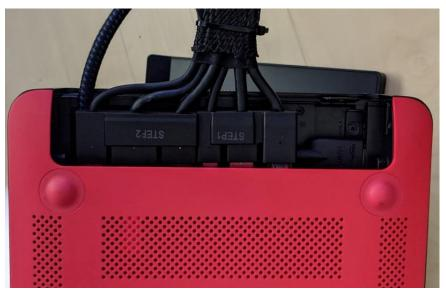
5. Keeping the device on its side with the ports/cables facing up, slide the red cover along One Cable, align HDMI ingest cable to the notch and snap cover into place. You may find it easier to hold the cables in one hand while sliding the cover with the other hand.
