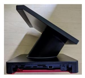
2. Insert an HDMI cable into HDMI Ingest port on inner right sidewall of base, lace it through the security channel and set it into the rounded notch.
