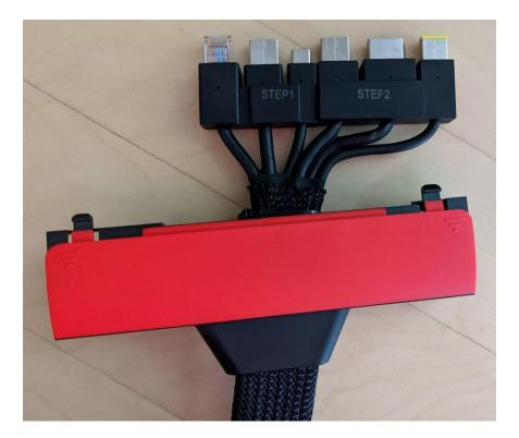
4. Align the connectors labeled 'Step 1' and 'Step 2' to the ports on the base. Gently push the connectors into the corresponding ports, moving from right to left.
