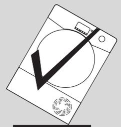
If the product is in different side, wait at least 4 hours before switching on so that the oil can flow back into the compressor. Failure to do this could result in damage to the compressor.
