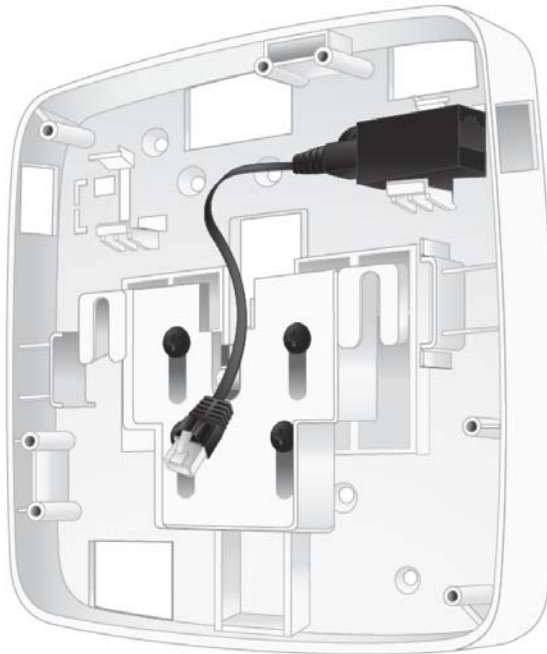
Figure 3 Inserting Ethernet cable into RJ45 coupler
