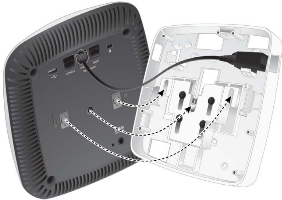
Figure 4 Securing the access point to the mounting bracket
