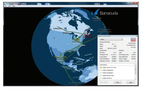
Barracuda NG Earth is a graphical real-time 3D network monitoring utility that provides a status overview of all VPN site-to-site tunnels.
