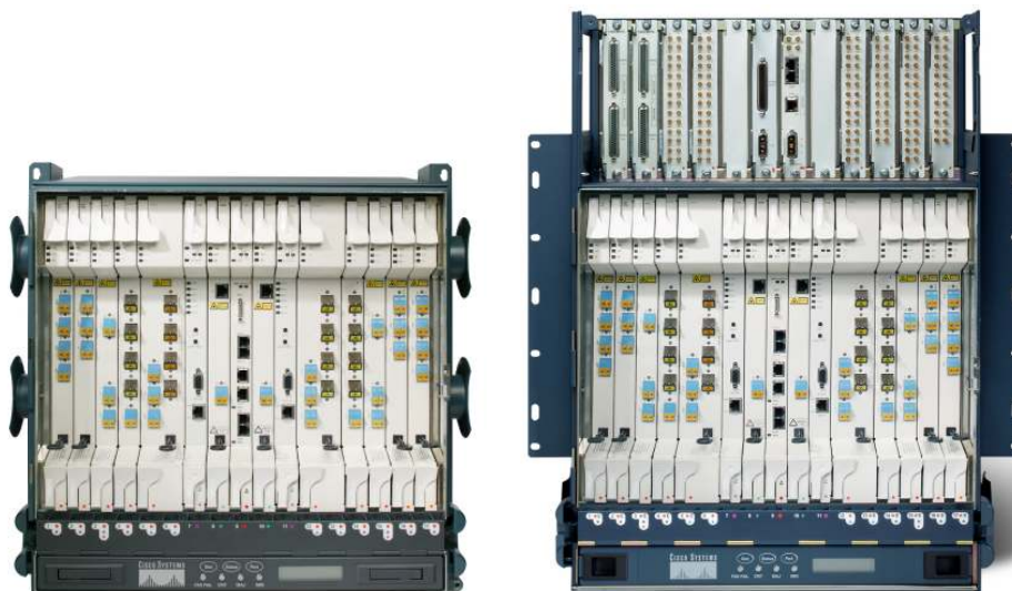
Figure 1. Cisco ONS 15454 Multiservice Transport Platform – ANSI (left) and ETSI (right) mechanics
