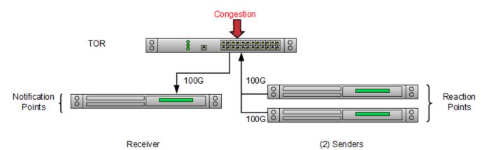
The two main components that determine the congestion control efficiency are the marking policy at the switch and the sending NIC behavior. The set of rules for the behavior of the sending NIC when there is congestion and when there is not, is the congestion control algorithm.
