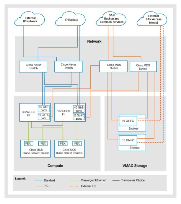
The following figure shows a network block storage configuration for the VxBlock System 1000 with 32 Gb/s SAN switches:
