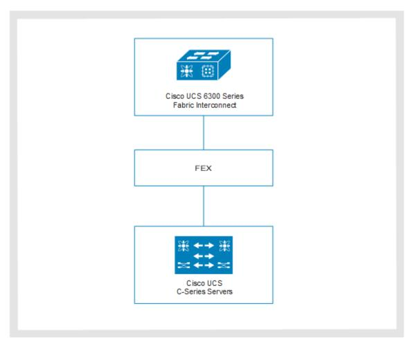
The following figure shows a configuration with a direct connection:
