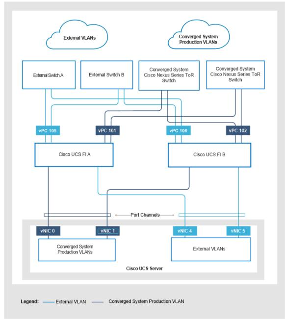
vPCs 101 and 102 are production uplinks that connect to the network layer of the Converged System. vPCs 105 and 106 are external uplinks that connect to other switches.
