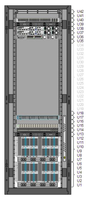
Patch Panel B Duct Cisco Nexus 31108TC-V Switch 1B Cable Management Cisco UCS C220 M5 server 1D Cisco UCS C220 M5 server 1C RecoverPoint Appliance 1-2 Support Shelf
