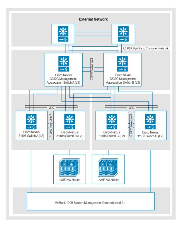
In this scenario, management network Layer 3 SVIs, and HSRP addresses can reside on the VxBlock System 1000 management aggregation switches or on the external network. There is one uplink from each Cisco Nexus 31108TC-V Switch to each Cisco Nexus management aggregation switch at 100 Gb/s.
