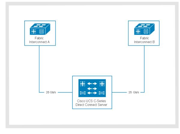
When a Cisco UCS rack server with Cisco UCS VIC 1455 is connected to a Cisco UCS 6454 FI through a 25 Gb/s cable, manually configure the server port. Port autodiscovery is not supported.
