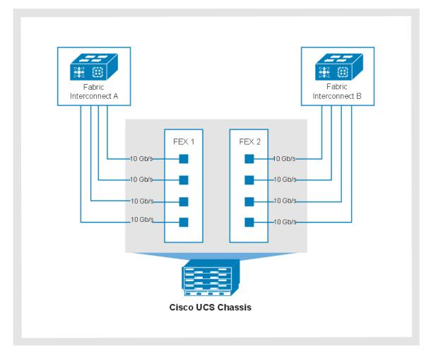
The following figure shows an eight-link IO module at 10 Gb/s port speed UCS Gen 4 IOM (2208) to Cisco UCS Gen 4 FI (6454) connections on a chassis:
