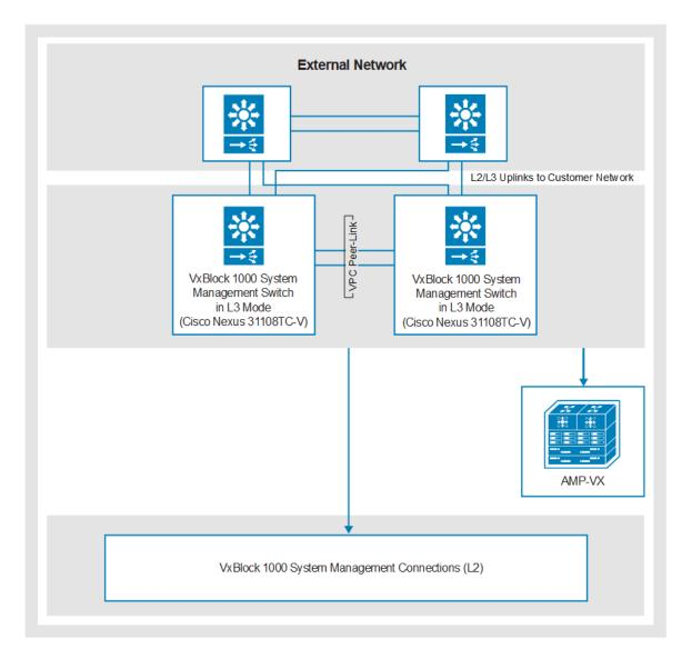
In this scenario, management network SVIs and HSRP addresses can reside on the VxBlock System 1000 management switches (Layer 3) or on the external network (Layer 2).
