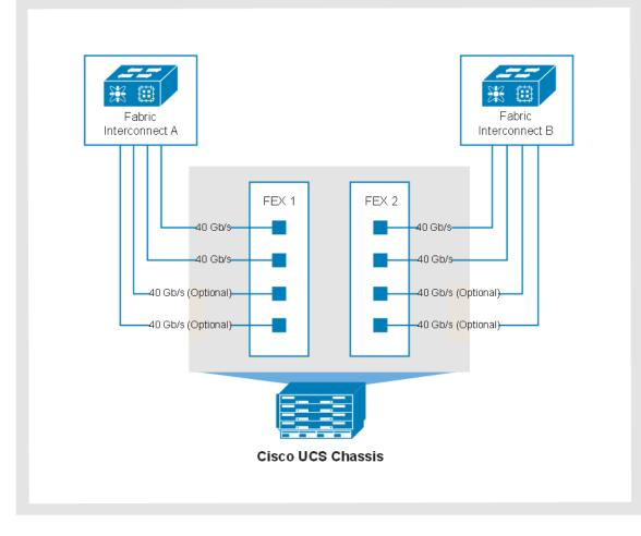
The following figure shows a four-link IO module to Cisco UCS Gen 4 FI connections on a chassis:
