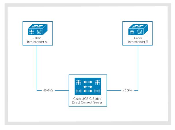
The following figure shows a direct connection between the Cisco UCS C-Series server and the Cisco UCS 6454 Fabric Interconnects:
