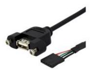
This 1ft USB to Panel mount USB cable features a 5-pin motherboard header connection on one end and a panel mount USB A (female) port on the other, providing a simple and easy to access USB 2.0 port on a panel mount receptacle.
